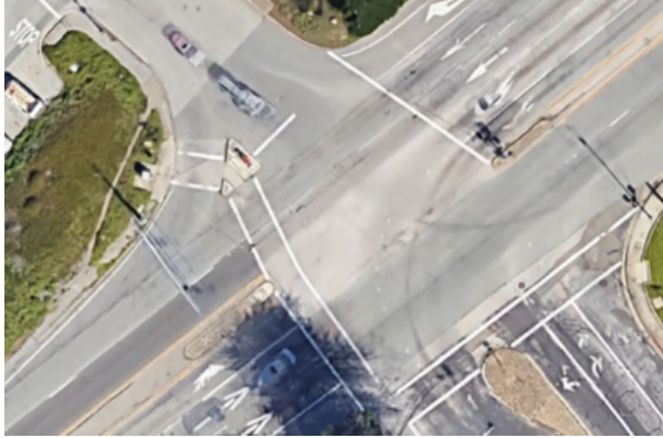
The Rockaway Beach/Fassler/Highway 1 intersection. There is a slip lane at the western approach feeding to Highway 1. – Image: GoogleMaps
